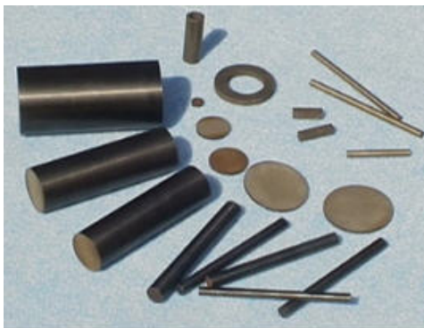
Magnetostrictive alloy composed of terbium, dysprosium, and pure iron
